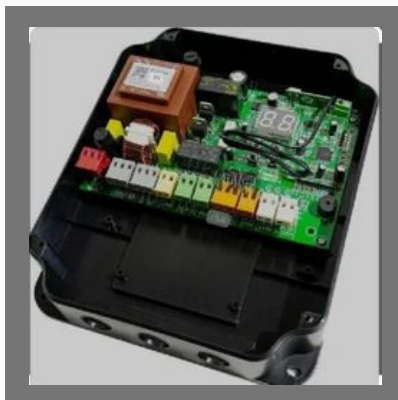
Control Card For Sliding Gate Motors
